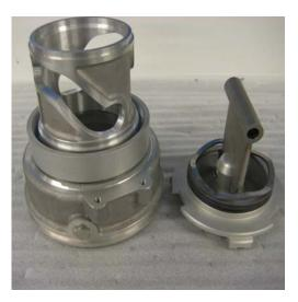
Before the coupling body places on the driving plate packet, make sure that the part where the upper cam curve ends, shall be placed exactly over one roll, and the heel on the driving plate packet should be placed under the hole for the shaft.
