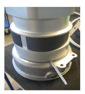
Place the swivel sleeve over the coupling body and screw in the swivel sleeve.
