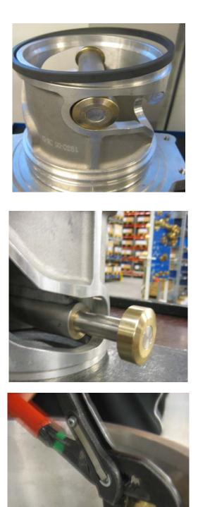
Change the Teflon® ring (pos.25) on the top of the coupling body.
