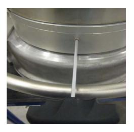
Begin with unscrewing and remove the lock screw from the swivel ring.
