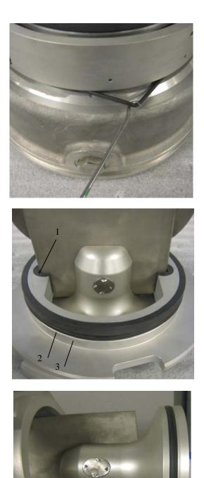
If necessary change O-ring (pos.21) for dust –protection. Use grease on the new O-ring.
