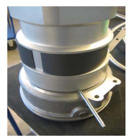
Mark the position of swivel sleeve against swivel ring with an Ø8 mm pin.
