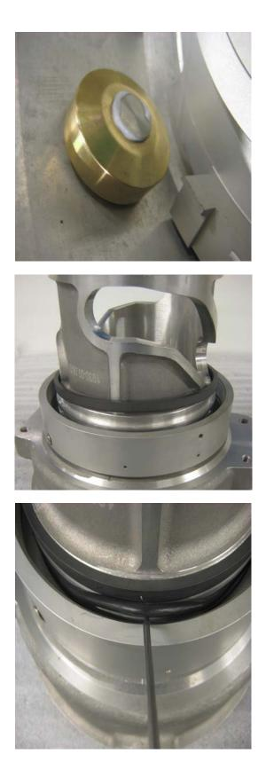
Change the three shafts (pos.18) and rollers (pos.17) to new ones.
