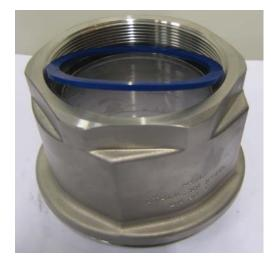
Place a new flat seal (pos.29) on the swivel sleeve. (Not needed when NPT-thread)
