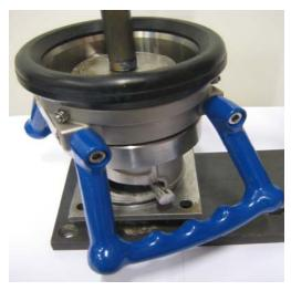
Remove the two shafts for piston guide, by applying pressure to the driving plate packet so that it moves down 2 mm. So that the drivning plate packet is released from the rollers.
