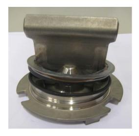
Change the O-ring (pos.8) and Teflon® ring (pos.9) on the driving plate back side. Use grease on O-ring.
