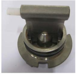
Change the Teflon® bushing (pos.16) to new ones on both sides.
