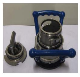
Before the coupling body places on the driving plate packet, make sure that the part where the upper cam curve ends, shall be placed exactly over one roll, and the heel on the driving plate packet should be placed under the hole for the shaft.
