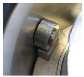
Press down and turn the driving plate to the position where the driving plate heels are placed under the rollers.
