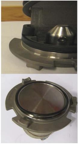
Change the Teflon® bushing (pos.13) to new ones on both sides.
