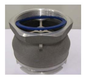
Assemble a new flat sealing (pos.12).
