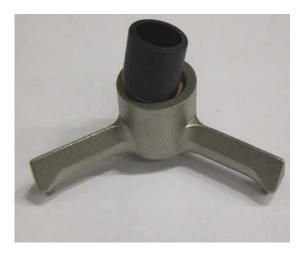
Replace the Teflon® bushing (pos.5) in the spindle steering with a new one.
