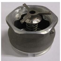
Press down the spindle steering and turn, to fix it in its position.
