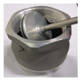
To take out the piston put into a relaxing position in the valve seat.
