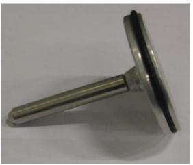
Replace the O-ring (pos.3) on the piston with a new greased O-ring.
