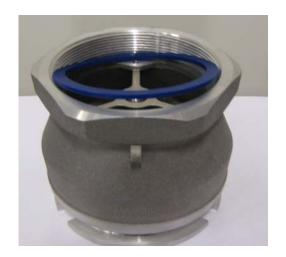
Remove the flat sealing.
