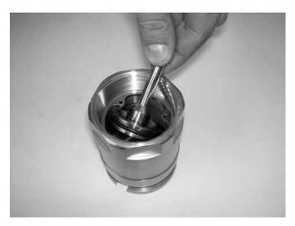
Put the piston into a relaxing position in the valve seat.
