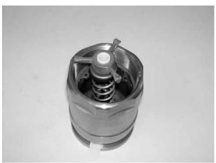
Replace the spring (pos.7), springcap (pos.6) and the spindle steering (pos.4).
