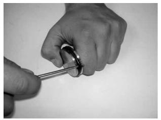
Replace the O-ring on the piston with a new greased O-ring (pos.3).
