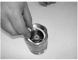
Assemble a new flat sealing (pos.12). NPT-thread does not have a flat sealing. Finally, make a visual inspection that everything is in its right place. Do also a test connection/disconnection with a hose unit that not is mounted and not has any fluid inside. If the coupling works all right you are ready to use it again.
