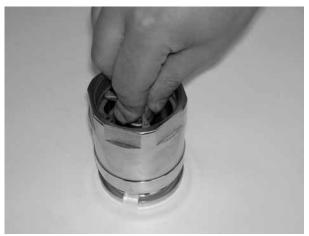
Press down the spindle steering and turn it free.
