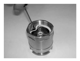
Remove the flat sealing NPT-thread doesn't have a flat sealing. Make sure you don't scratch the seal face.
