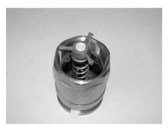
Take out all the parts from the body (spindle steering, springcap, spring, piston).
