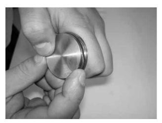
Have an equal pressure around the O-ring. The O-ring must be pressed into the groove on the piston.
