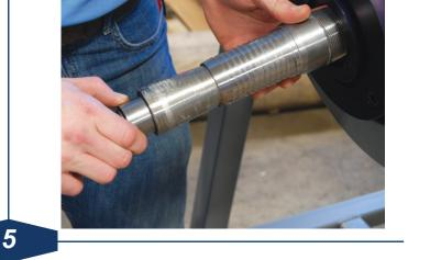
Accurately measure the hose O.D. with a diameter tape. Select the correct IX ferrule from the DPL based upon the hose O.D. just measured. Note: Always measure both hose ends for accurate ferrule selection.
