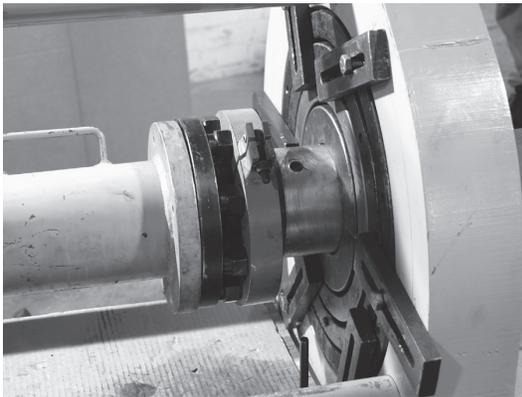
Move the directional control lever to the "Forward" position and depress the button on the remote. Advance the cylinder forward until the end of the ferrule is near the die opening. Using a wooden board or metal pipe, lift the ferrule up. Jog the cylinder by depressing and releasing the button on the remote. This will allow the ferrule to enter the die slowly. After the ferrule has entered the die, stop advancing the cylinder.
