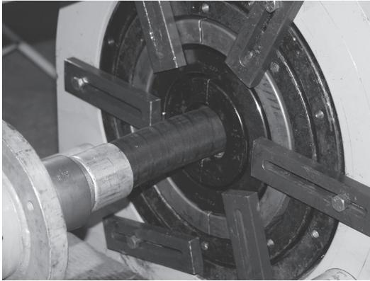
While holding the die in place with one hand, place one of the tie down bars over the die so that it does not come out of the die holder unexpectedly. Secure the tie down bar by tightening the bolt.
