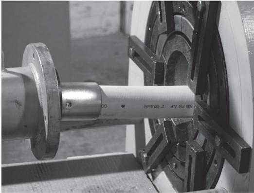
Lifting up the hose, insert one die half under the hose. Lower the hose so that it rests on the die. Insert the other die half. Make sure that the seams of the die do not line up with the seams on the die holders.
