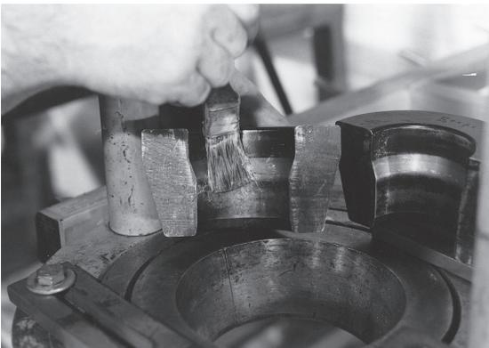
Lubricate the I.D. of both die halves with Crisco® (recommended) or high viscosity oil or heavy duty grease.
