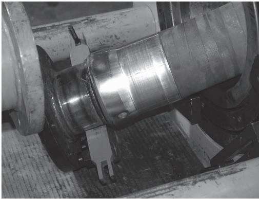
Position a rubber sheet or pad under the die bed. *Slowly* slide the hose towards the pusher. When the die clears the die holder, one or both halves may fall to the floor. If one half remains on the ferrule, tap it with a mallet until it releases. If both halves remain on the ferrule, it may require the halves be pried apart at the seam.
