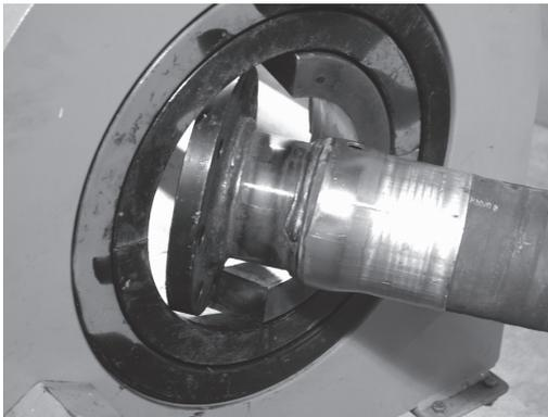
Loosen the bolt(s) on the tie down bar(s) and move the tie down bar(s) so that they clear one die bed spacer. Tighten any bolt just loosened. Remove the die bed spacer one half at a time. Repeat this process for each die bed spacer to be removed. Remove only enough die bed spacers to allow the flange to pass through.
