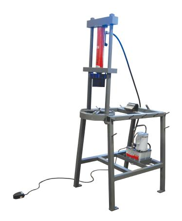
**Dixon** 800 High Street • Chestertown, MD 21620 ph: 877•963•4966 fax: 800•283•4966 *dixonvalve.com*  Before you begin, make sure the ram is fully retracted. Install **25PUSH400** (also referred to as the pusher hat) onto the main pusher plate. Install the **MISCPUSH** into the **25PUSH400** and secure with set screw.
