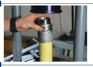
Install the proper pusher onto the stem. (Reference the chart for proper pusher selection)
