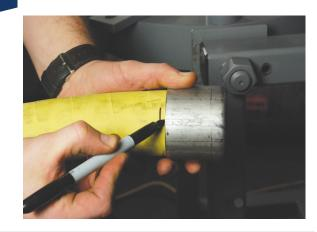
Slide the ferrule onto the hose. Place a mark on the hose at the end of the ferrule. Move the ferrule 1/8" from the mark just made towards the end of the hose. Place a second mark on the hose at the end of the ferrule.
