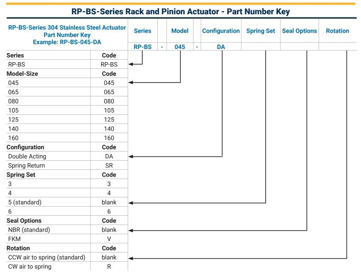
RP-BS-Series Rack and Pinion Actuator - Spring Set Kit Part Number Key
