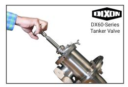
Our unique easy-lock plunger does not require external locking devices to lock the plunger open during transfer. Instead, pull the plunger open and rotate the handle to engage the internal lock. No stem clip cotter pin needed.
