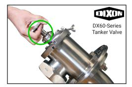
With the plunger in the fully closed state, there is 1-3/8" of clearance between the handle and bonnet on Dixon's DX60-series tanker valve. This eliminates the finger or hand entrapment point present on competitor valves.
