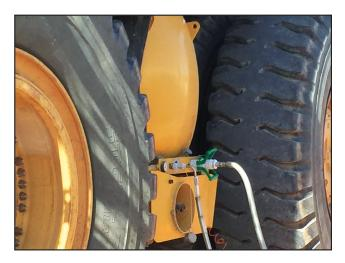
LNG fueling application on off-highway mining truck
