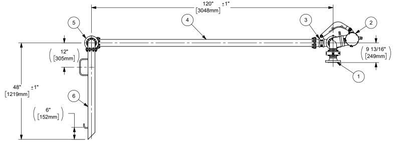
PRODUCT TO BE CONVEYED: ASPHALT SWIVEL SEALS (CONTACTING PRODUCT): FKM GREASE: STANDARD (LITHIUM SEMI-SYNTHETIC)
