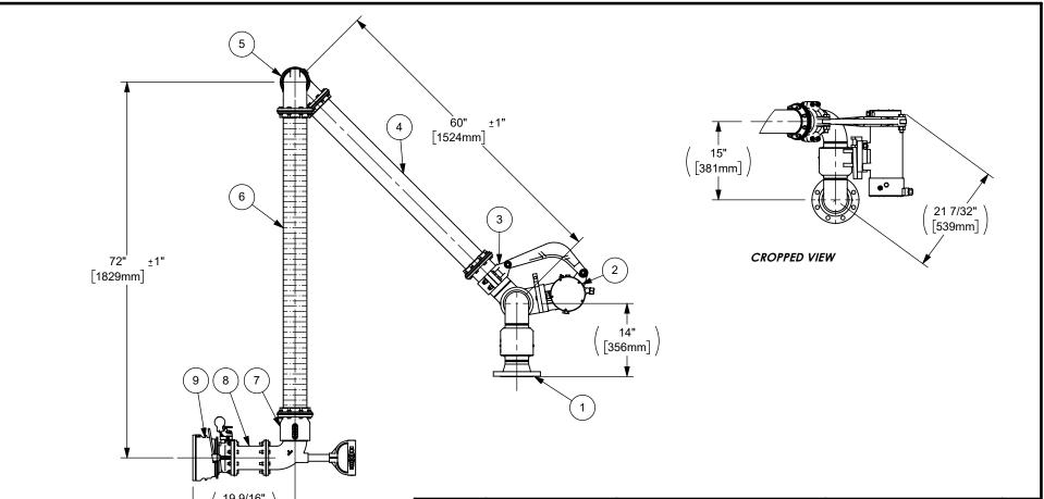
SWIVEL SEALS (CONTACTING PRODUCT): FKM GREASE: STANDARD (LITHIUM SEMI-SYNTHETIC)
