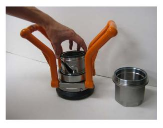
Change the Teflon® ring (pos.25) on the top of the coupling body.
