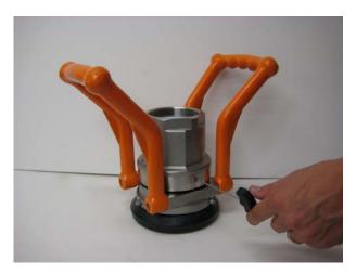
Begin with unscrewing and remove the lock screw from the swivel ring.
