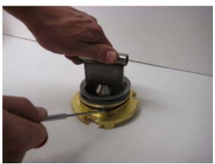
Change the O-ring (pos.8) on the driving plate back side. Use grease on O-ring.
