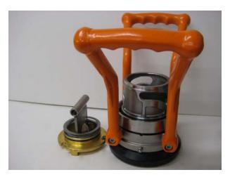
Before the coupling body places on the driving plate packet, make sure that the part where the upper cam curve ends, shall be placed exactly over one roll, and the heel on the driving plate packet should be placed under the hole for the shaft.
