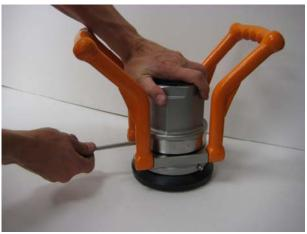
Mark the position of swivel sleeve against swivel ring with an Ø8 mm pin.
