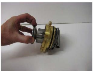
Press down the O-ring with your thumb. Make sure that the O-ring fits into the groove.
