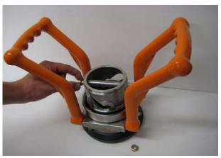
Assemble the two shafts for piston guide.
