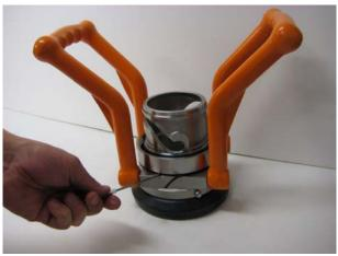
Change the O-ring (pos.24) from the groove in the coupling body.
