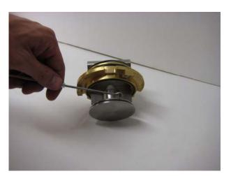
Change the O-ring (pos.3) on the piston. Use grease on the new O-ring. Make sure that the O-ring doesn't get twisted when mounting.
