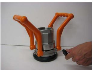
Use Loctite® 243 and screw the lock screw into the swivel ring without any force! Risk to deform the ball bearing!
