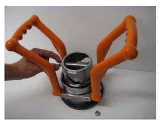
Remove the two rollers and the rolling shaft from the piston guide.
