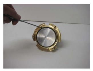
Change the O-ring (pos.6) on the driving plate front side. Use grease on O-ring.
