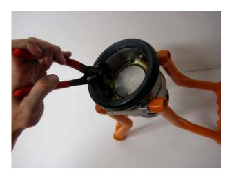
Press down and turn the driving plate to the position where the driving plate heels are placed under the rollers.
