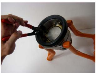
Turn the driving plate to the position where the recess ends up under the rollers under pressure to the driving plate packet.
