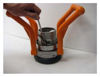
If necessary change O-ring (pos.21) for dust –protection. Use grease on the new O-ring.
