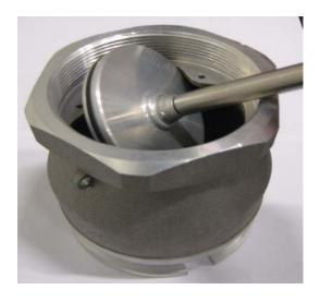
To insert the piston back again it should be putted in a relaxing position in the valve seat
