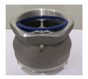
Remove the flat sealing.
