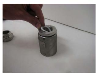
Drop the balls into the swivel joint, turn the swivel sleeve after each ball.
