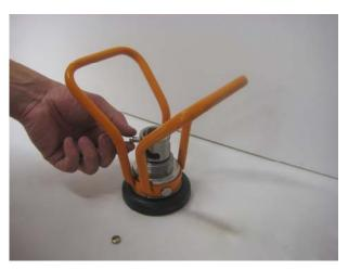
Put the shafts for piston guide and the rollers in their position in the piston guide.
