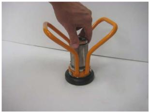
Remove the coupling body from the swivel sleeve.
