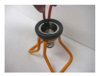
Press down the piston and turn the driving plate to the position where the recess ends up under the rollers.
