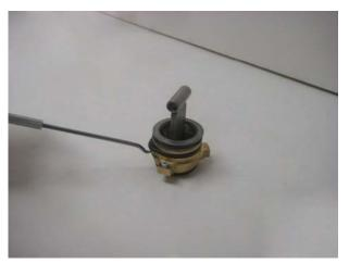
Remove the O-ring and replace with a new O-ring (pos.8). Use grease on the O-ring.
