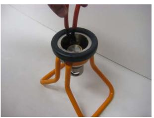
Before the coupling body places on the driving plate packet, make sure that the part where the upper camcurve ends, shall be placed exactly over one roll, and the heel on the riving plate packet should be placed under the hole for the shaft. Press down the piston and press together the driving plate with the roller, so they are in position Tools: Arbor, Polygrip plier
