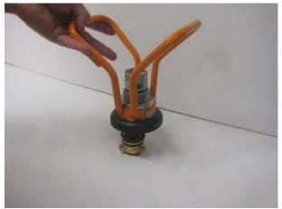
Remove the driving plate packet from the body.
