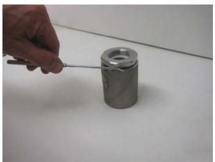
Remove the O-ring from the swivel sleeve.
