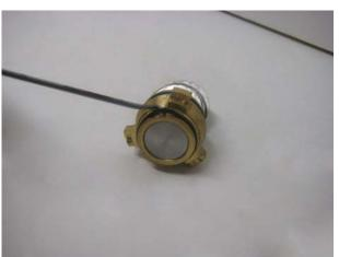
Remove the O-ring and replace with a new O-ring (pos.6). Use grease on the O-ring.
