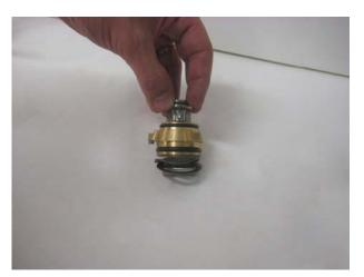
Assemble the driving plate packet with the body.
