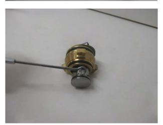
Remove the O-ring and replace with a new O-ring (pos.3). Use grease on the O-ring.
