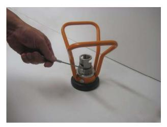
Change the O-ring (pos.33) on the coupling body; use grease on the O-ring.
