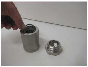
Change the O-ring (pos.24) to a new one; apply grease on the new O-ring.
