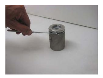
If necessary change O-ring (pos.21) for dust –protection. Use grease on the new O-ring.
