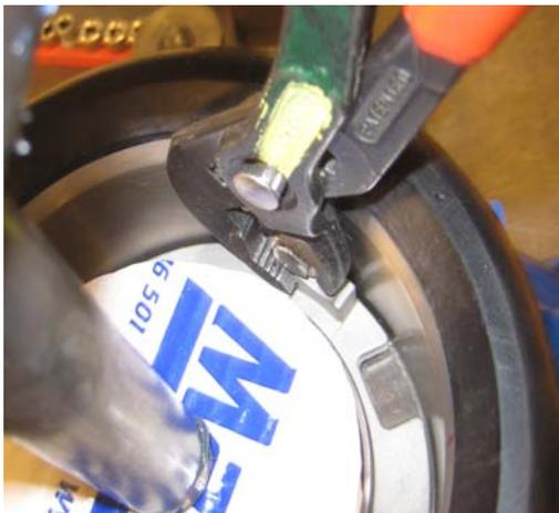
Turn the driving plate to the position where the recess ends up under the rollers under pressure to the driving plate packet.
