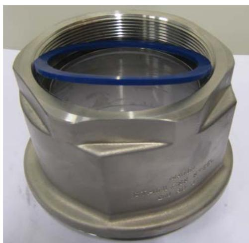
**Place a new flat seal (pos.29) on the swivel sleeve. (Not needed when NPT-thread)**
