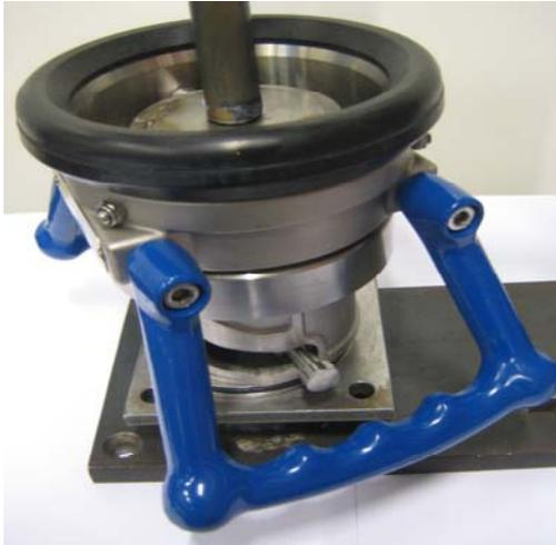
Remove the two shafts for piston guide, by applying pressure to the driving plate packet so that it moves down 2 mm. So that the driving plate packet is released from the rollers.
