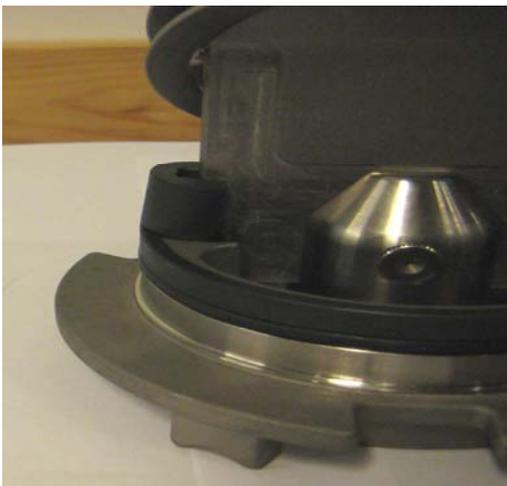
**Change the Teflon® bushing (pos.13) to new ones on both sides.**
