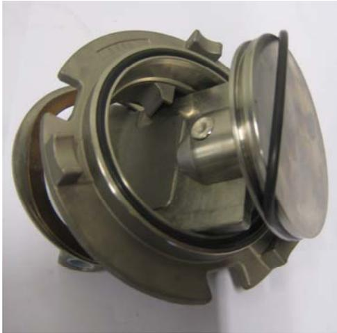
**Change the O-ring (pos.3) on the piston. Use grease on the new O-ring. Make sure that the O-ring doesn't get twisted when mounting.**
