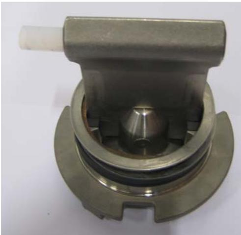
**Change the Teflon® bushing (pos.16) to new ones on both sides.**
