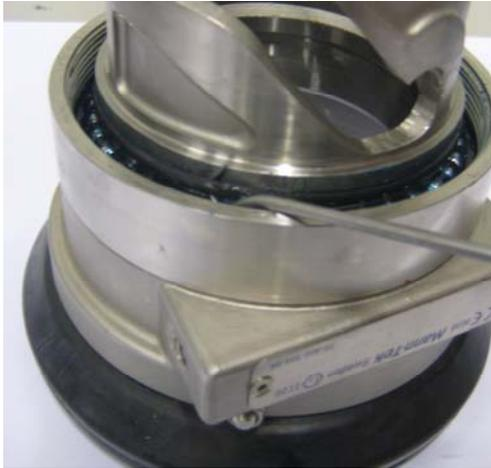
Remove and change the O-ring (pos.24) from the groove in the coupling body. Use grease on the new part. Apply grease on the balls for best possible swivel rotation.
