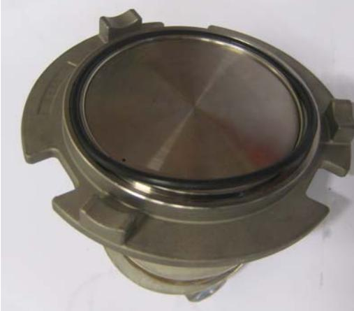
**Change the O-ring (pos.6) on the driving plate front side. Use grease on O-ring.**
